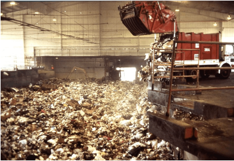
SAN FRANCISCO POST-RECYCLING SOLID WASTE AT TRANSFER STATION. NOTE THE LARGE LOADING CRANE AT THE FAR END OF THIS PIT.
